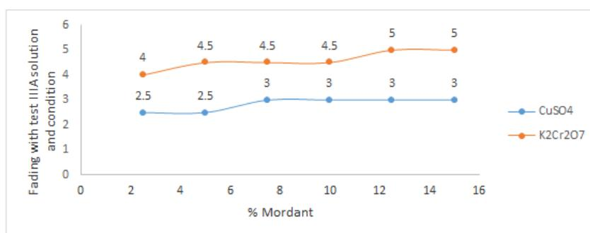
**Fig-2: Effect of test solution IIIA and condition to washing/ staining fading of dye from wool fabric**
