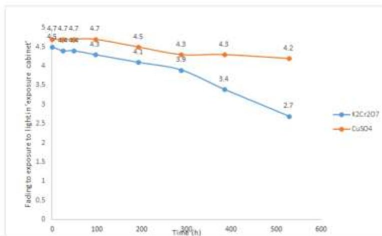
**Fig-3: Effect of exposure to light on fading of dye from fabric after 528 hours (22 days)**
