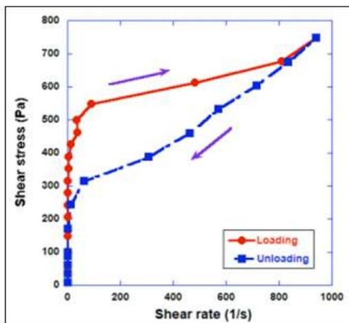
**Fig-1: Typical flow curves of mortar with the addition of 0.29% of polymer**
