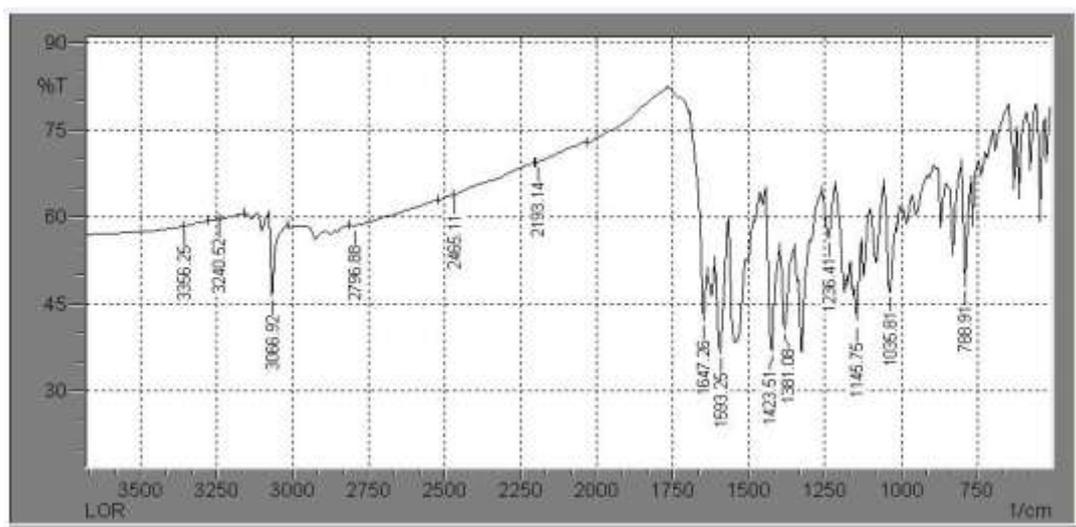
Fig-5: Infrared spectrum of Lornoxicam
