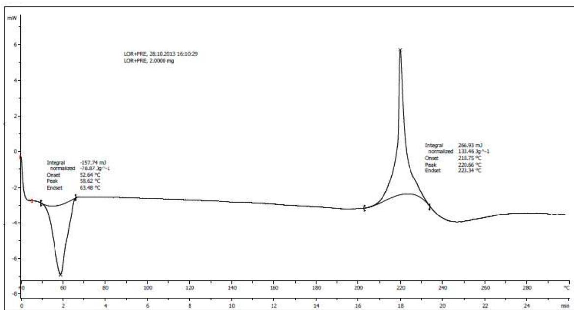
Fig-4: DSC thermogram of physical mixture containing Lornoxicam and Precirol in 1:1 ratio
