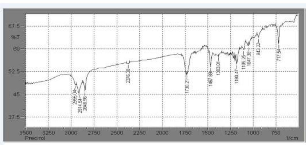
Fig-6: Infrared spectrum of Precirol
