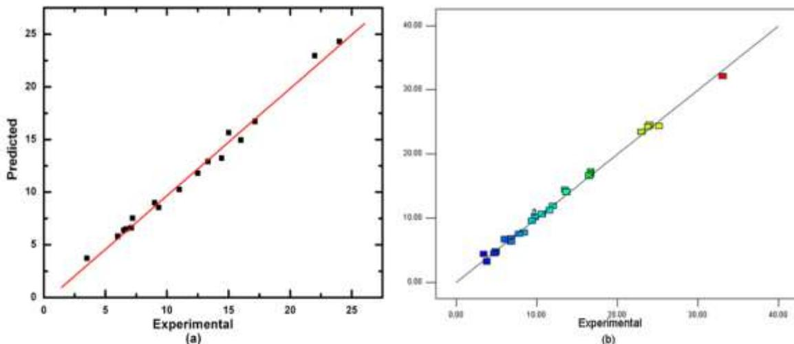
Fig. 3: Comparison between the experimental and the predicted values of dimensionless bed pressure drop by (a) dimensional analysis and (b) statistical analysis
