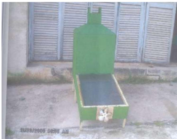
Fig. 2 b. Constructed indirect solar dryer
