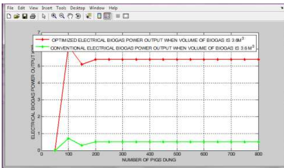
Fig-4: Comparing optimized electrical biogas power output with the conventional method when volume of the biogas 3.6m 3 respectively
