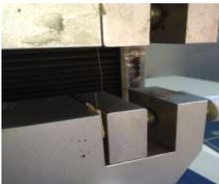
**Fig-3: Single strand after testing**
