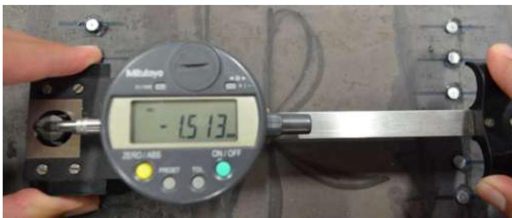
Fig-8: Photograph showing measurement between dots using the DEMEC device
