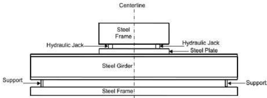
Fig-1: Layout of the frame and cambering equipment [1]
