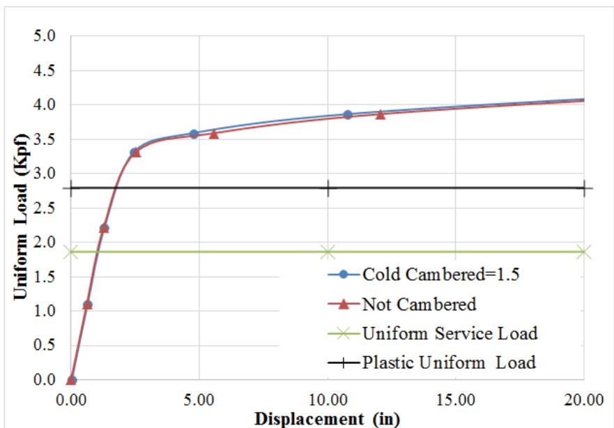
Fig-12: Load-displacement of W8X18-CC-1.5-PP and non-cambered beams
