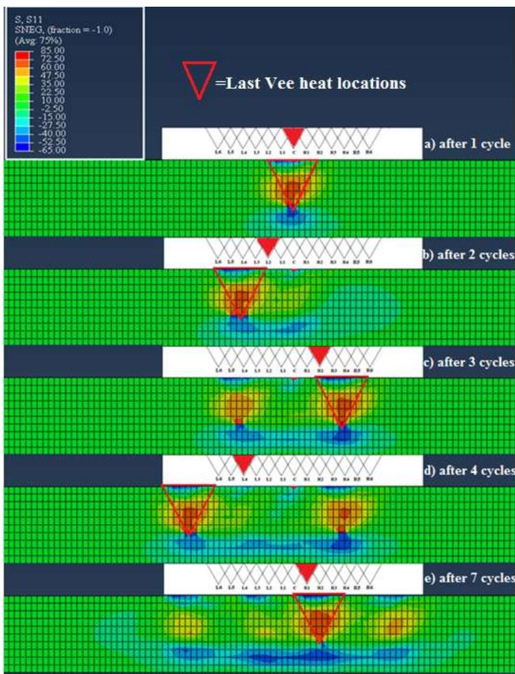
Fig-15: Web longitudinal residual stresses in the first W8X18 beam after various heating cycles
