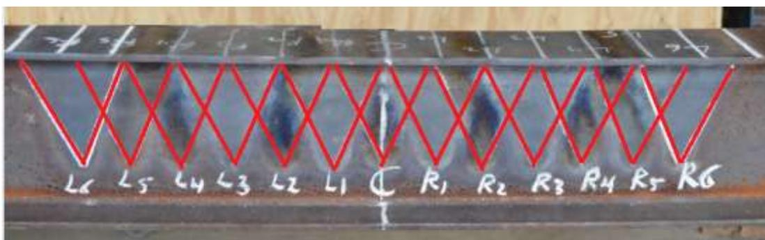
Fig-5: Nomenclature/location of Vee heats applied to W8X18 beam specimen
