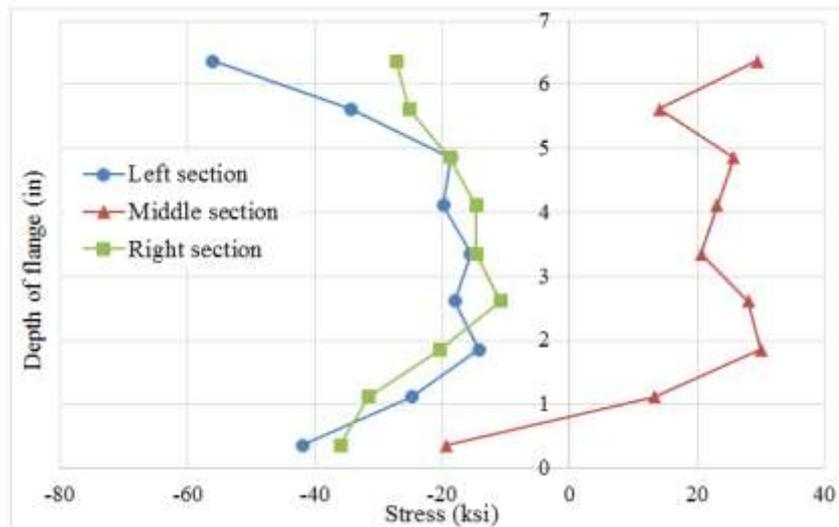
Fig-10: Residual stresses in the top flange of the W14X30 heat-cambered beam
