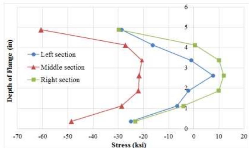
Fig-10: Residual stresses in the top flange of the W8X18 heat-cambered to 0.82 in
