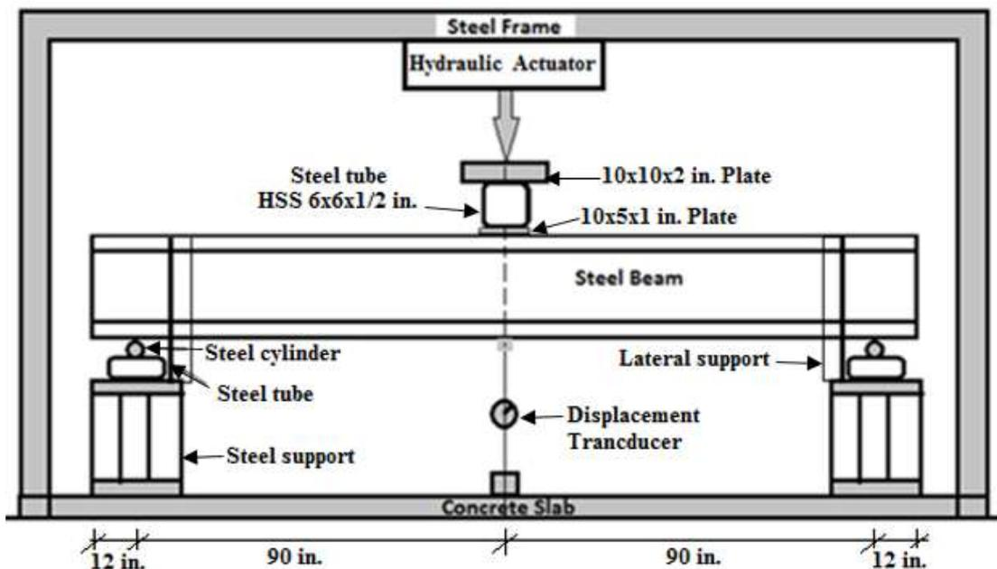
Fig-2: Experimental setup for cold-gambered beams
