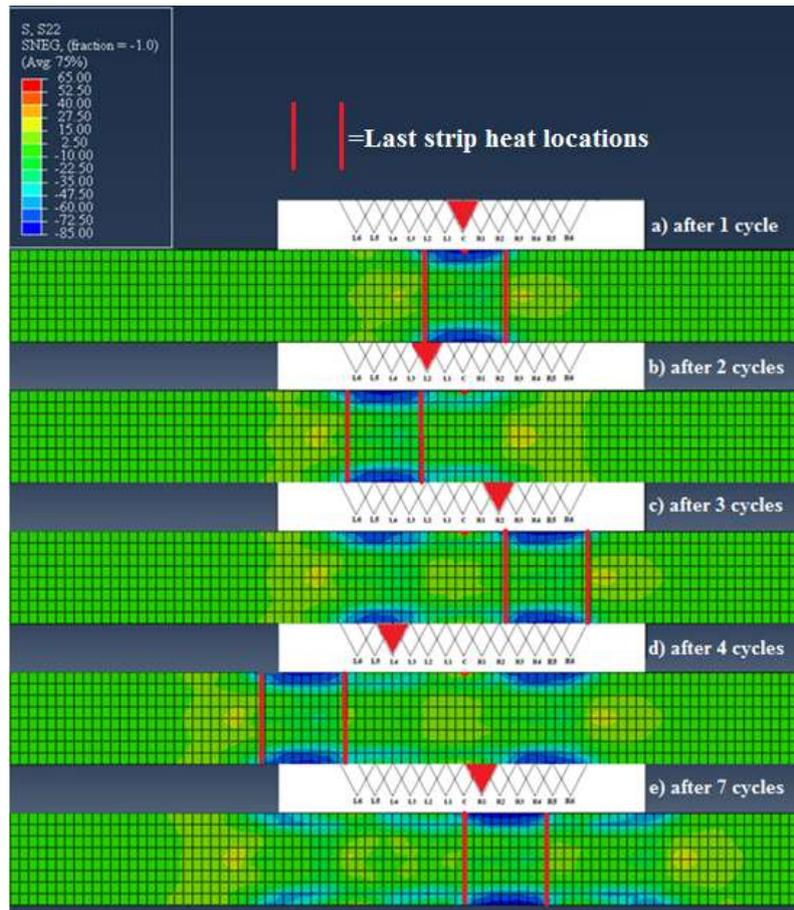
Fig-16: Top flange longitudinal residual stresses in the first W8X18 beam after various heating cycles
