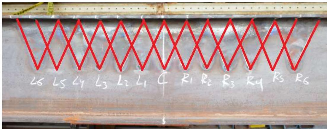
Fig-6: Nomenclature/location of Vee heats applied to W14X30 beam specimen
