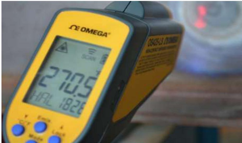
Fig-4: Infrared temperature gun used to measure steel temperature
