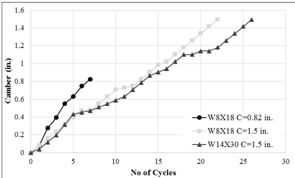
Fig-7: Relationship between the heating cycles and the total camber
