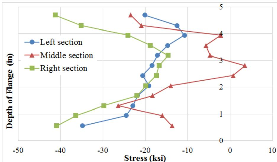
Fig-8: Residual stresses in the top flange of the W8X18 heat-cambered to 1.5 in.
