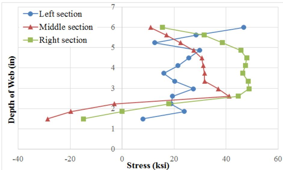
Fig-11: Residual stresses in the web of the W8X18 heat-cambered to 1.5 in
