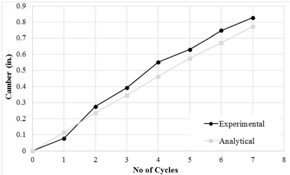
Fig-11: Analytical and experimental camber results for the first W8X18 beam
