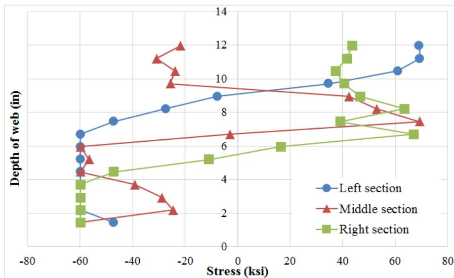
Fig-9: Residual stresses in the web of the W14X30 heat-cambered beam
