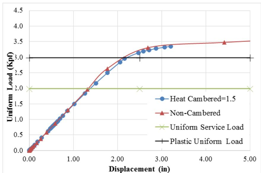
Fig-19: Load-displacement of W8X18-HC-1.5-PP and non-cambered beams
