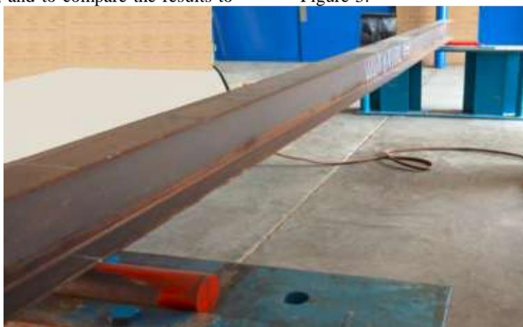
Fig-3: Test setup for heat-cambered beams on loading dock of STC
