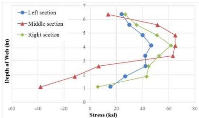
Fig-9: Residual stresses in the web of the W8X18 heat-cambered to 0.82 in
