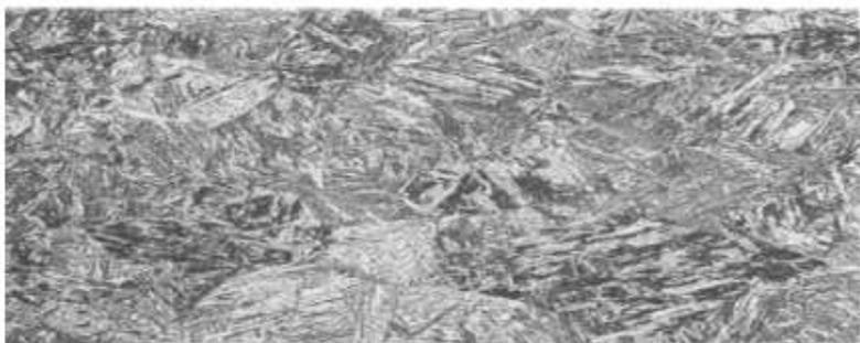
Fig-7: Microstructure of a typical martensite at 200x [6]
