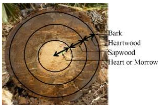
Fig-2: A cross section of the trunk of the Malfana’s palmyra tree [9]
