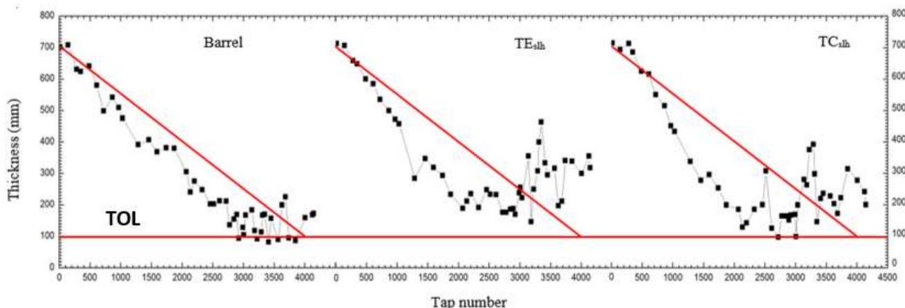
Fig-5: Screen example that shows the evolution of the Barrel,  $TE_{SLH}$  and  $TC_{SLH}$  lining thickness
