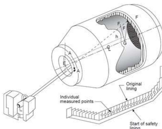
Fig-1: Scheme of the measurements practice with the laser scanner equipment [8]
