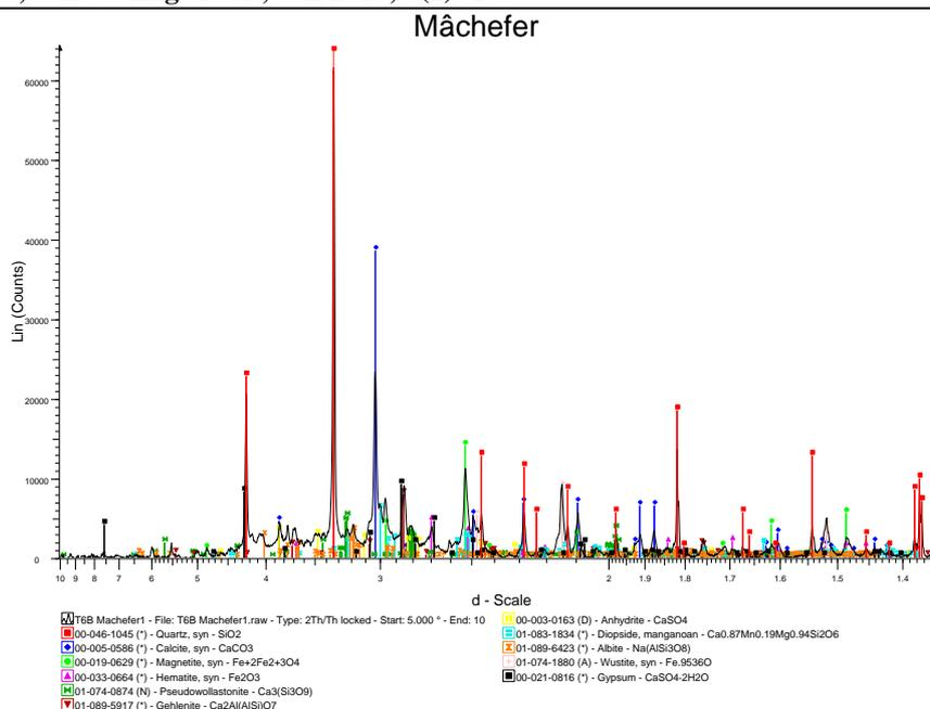
**Fig-4: Analysis by X-Rays Diffraction**
