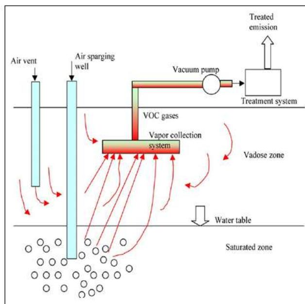
**Fig-3: Schematic of a Bioventing System [6]**
