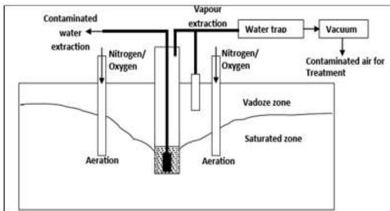
**Fig-4: A schematic diagram for vacuum extraction procedure [8].**
