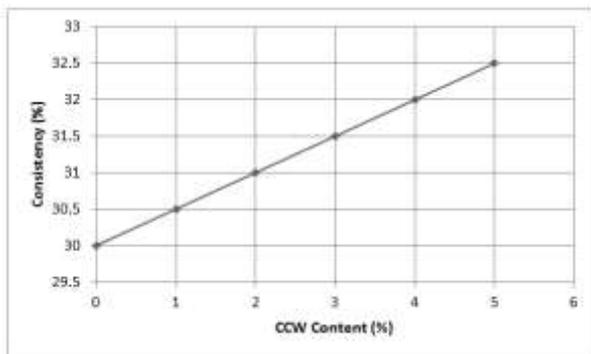
Fig-2: Normal consistency of Cement-CCW paste
