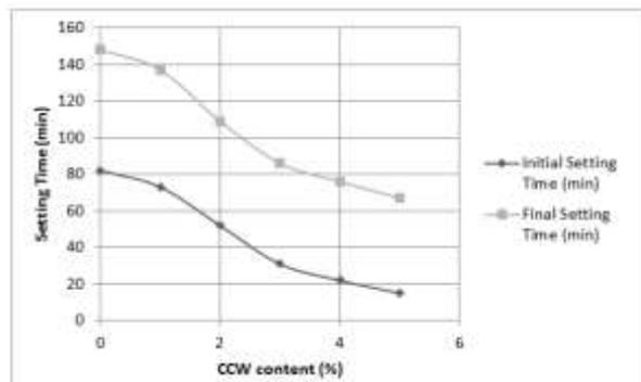
Fig-3: Initial and final setting times of Cement-CCW paste
