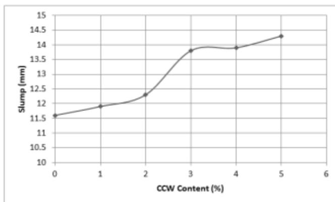
Fig-4: Slump of Cement-CCW fresh mortar
