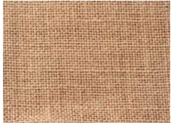
**Fig-5: Alkaline treated Jute Fiber**
