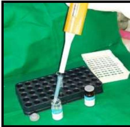
Fig-8: Addition of 50 $\mu$ l of chromogen reagent A, B to each well
