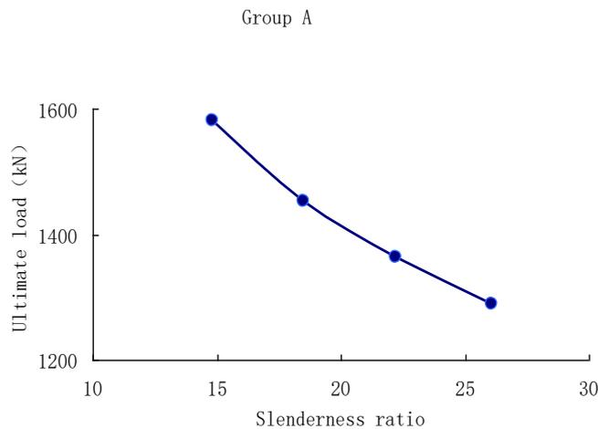
**Fig-2: A group slender ratio - limit load curve**
