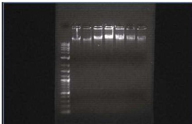
**Fig-1: Extracted DNA (lane 2 to 8) was tested on 1% agarose gel using 1 kb ladder (lane 1). Ladder shows 1000, 800, 700, 600, 500, 400, 300, 200, 100bp fragments**
