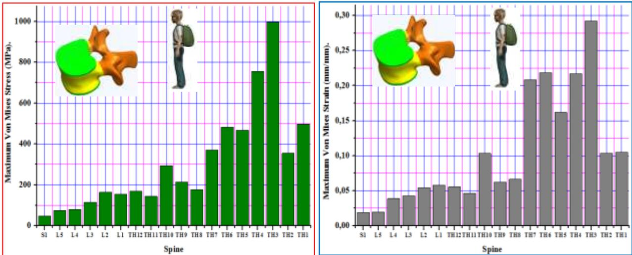
Fig-15: Histogram of stress and strain in the spine for a load of 20kg
