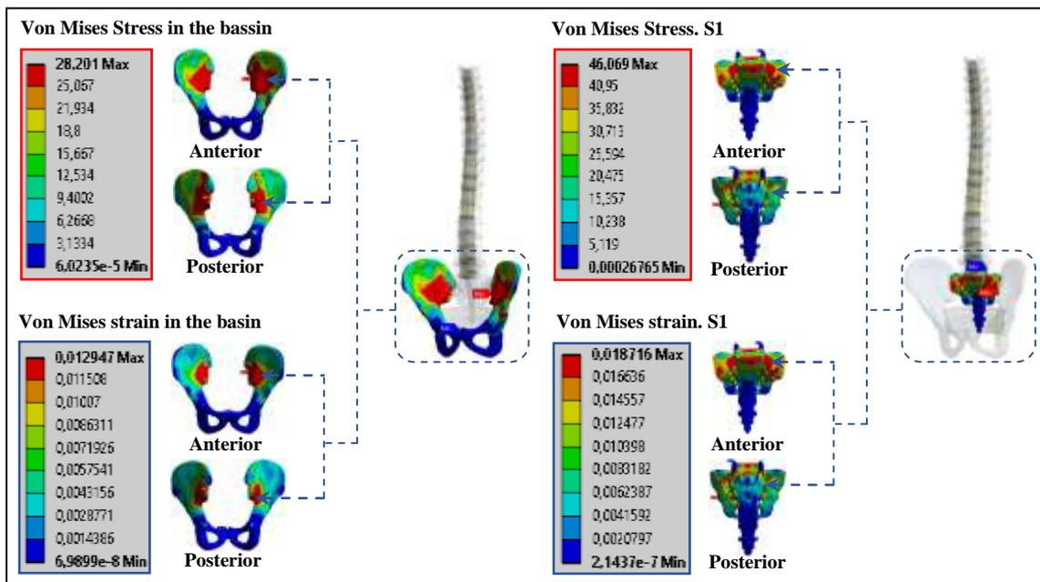
Fig-29: Distributions of stresses and strains in the basin and sacrum for a load of 20kg
