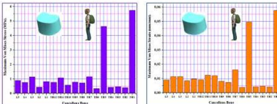
Fig-25: Histogram of stresses and strains in the cancellous bone with a load of 20kg
