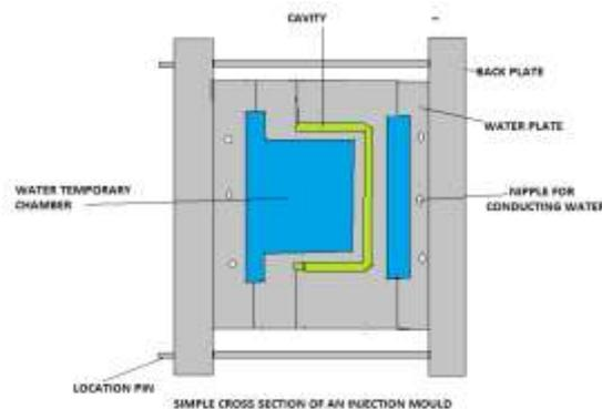
**Fig-3: mold basic parts**
