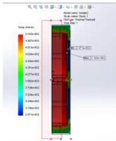
Fig-18: CROSS SECTION of the female mold
