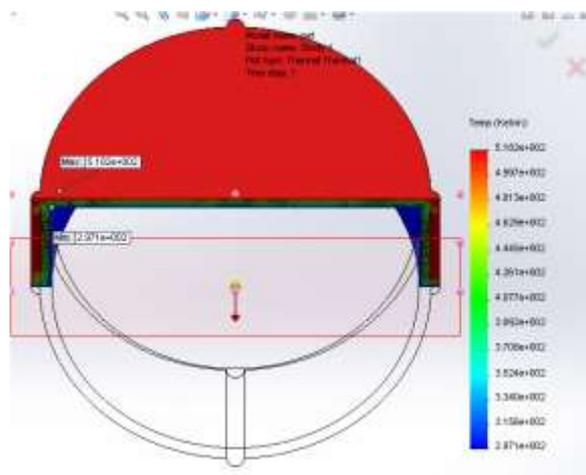
Fig-24: Simulated PET Product with Cooling Parameters Cross Section
