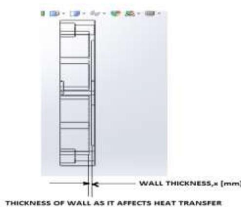
Fig-5: Heat analysis at the interface wall between mold cavity and cooling water cavity
