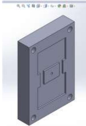
**Fig-13: 3-D Solid Model of Female Water Chamber**
