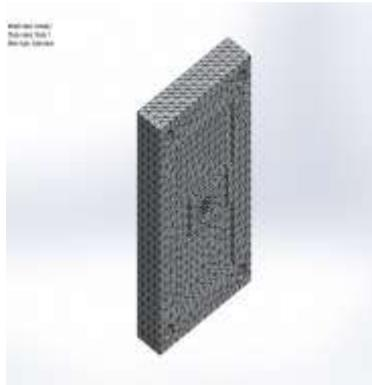
**Fig-14: solid mesh of the female mold (water cavity)**
