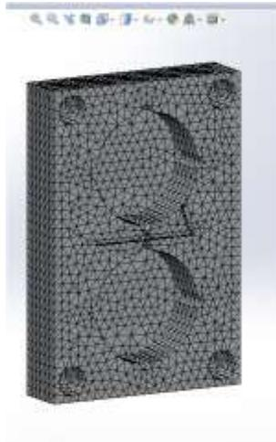
**Fig-15: Mesh of Female Mold Cavity**
