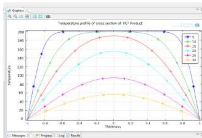
Fig-25: Temperature variation across of the thickness, x, mm of PET product
