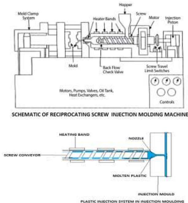
**Fig-2: screw conveyor injection system**
