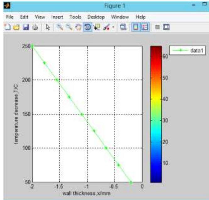
Fig-26: Cooling across the wall thickness of the mold
