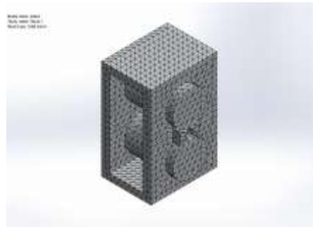
Fig-7: 3-D Solid Model of Male Mold Mesh
