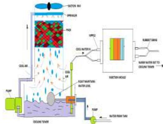
**Fig-1: A schematic diagram of an injection mold cooling system**
