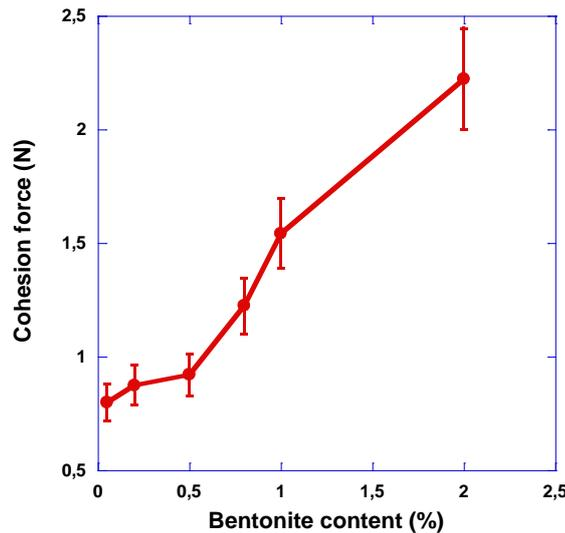
**Fig-4: Evolution of the cohesion force with bentonite content.**
