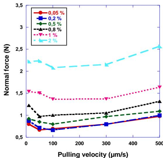
Fig-3: Evolution of the adhesion force as a function of the pulling velocity for varying bentonite contents.
