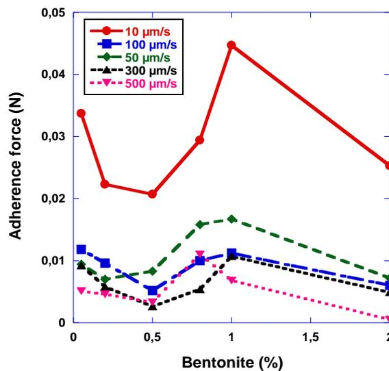
**Fig-5: Evolution of the adherence force versus bentonite content for different pulling velocities.**
