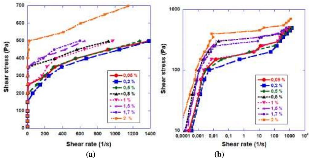
Fig-7: Flow curves obtained in rheological measurements of mortars in formulation with bentonite: (a) Linear scale; (b) Logarithmic presentation
