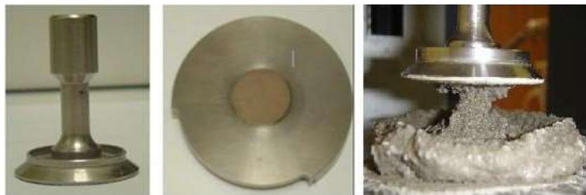
Fig-1. Tack geometries - Upper plate; Bottom plate; A tack test in process
