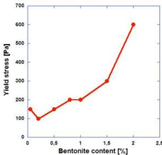
**Fig- 9: Evolution of the yield stress with bentonite content**
