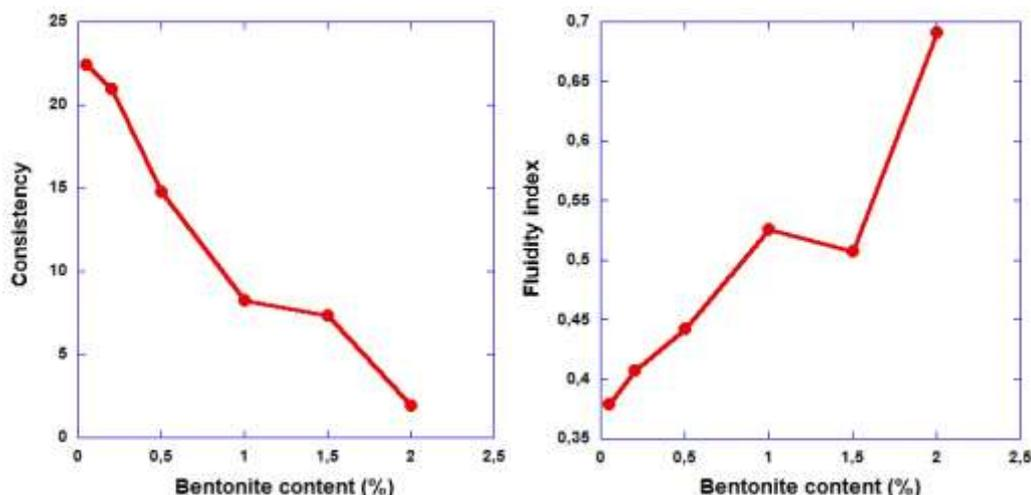
Fig-10: Evolution of consistency and fluidity index with bentonite contents
