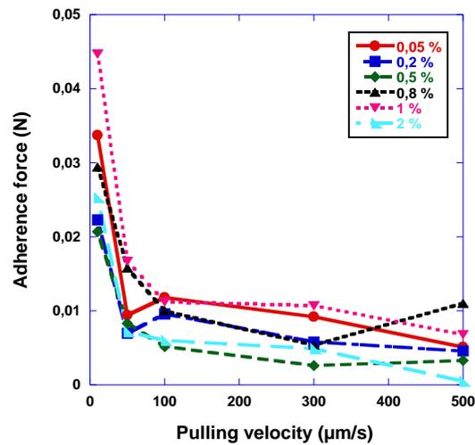
Fig-6: Evolution of the adherence force with pulling velocity for varying bentonite contents.
