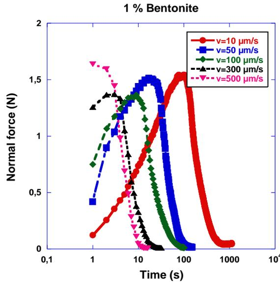
Figure 2: Evolution of pulling force for varying velocities for a mixture with 1% bentonite.
