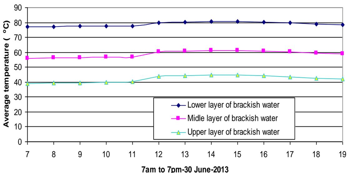
**Fig-1: The average temperature of wasterwater in solar pond in 30June 2013.**
