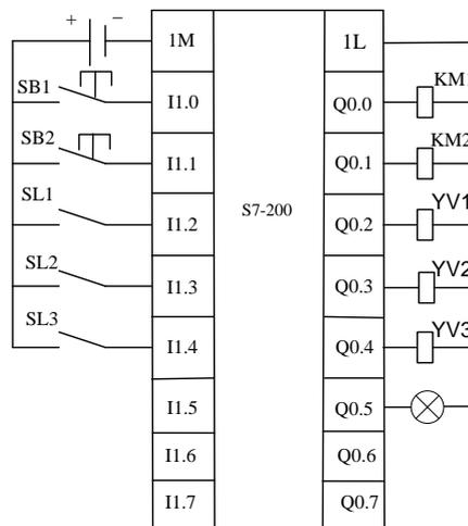
**Fig. 4: I/O wiring diagram of PLC**
