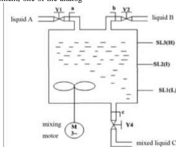
Fig. 1: The schematic diagram of system
