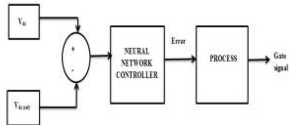
Fig. 8: Block Diagram of Neural Network based controller
