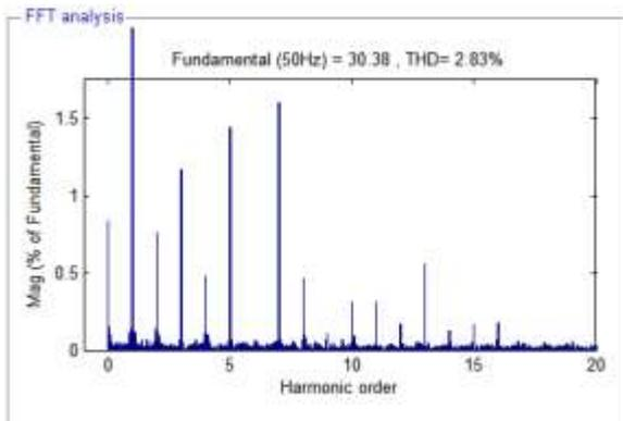
Fig. 15: FFT Analysis for Source Current using Anti-windup with Back calculation method
