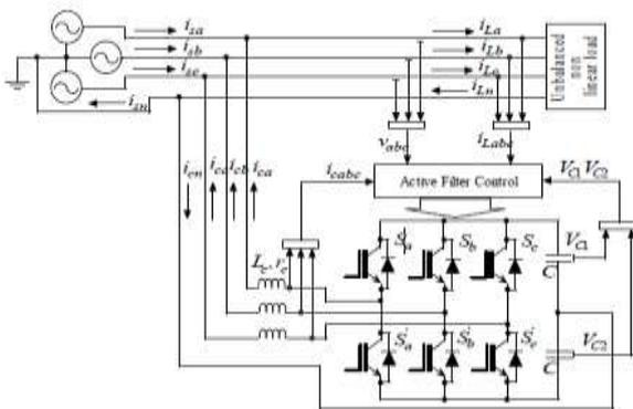
Fig.4: Structure of three phase four wire APF
