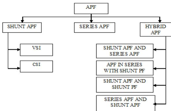
Fig. 1: APF Types based on power circuit configurations
