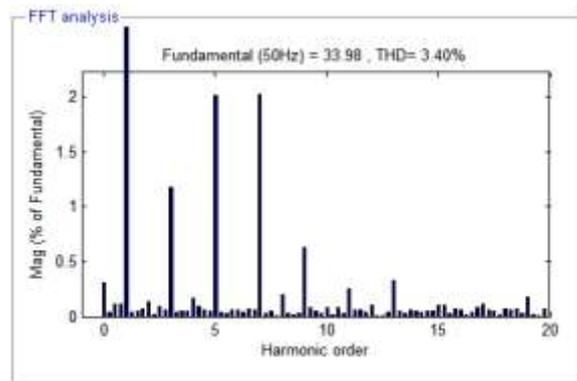
Fig. 12: FFT Analysis for Source Current using PI
