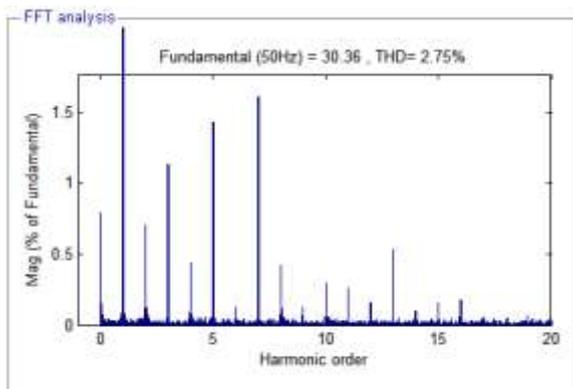
Fig. 16: FFT Analysis for Source Current using Anti-windup with tracking with Back calculation method
