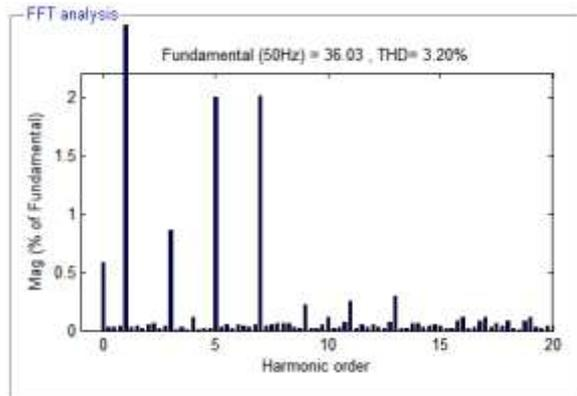
Fig. 13: FFT Analysis for Source Current using FLC
