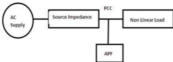
Fig. 2: Shunt APF configurations
