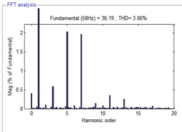
Fig.14: FFT Analysis for Source Current using ANN
