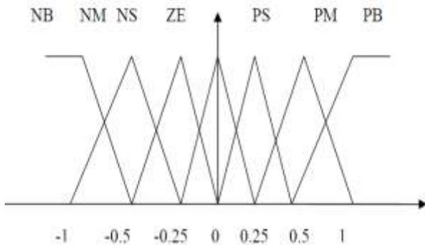
Fig.7: Membership function of fuzzifier input variables  $e, \Delta e$  and defuzzifier output variable  $\mu_a(x)$
