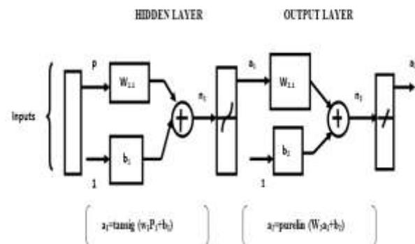
Fig. 9: Neuron model using Back Propagation
