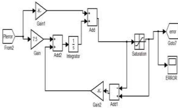
Fig.10: Block Diagram of Anti-windup using Back calculation method
