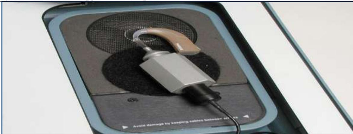
Fig-2: Experimental setup of BTE hearing aid attached to hearing aid analyzer
