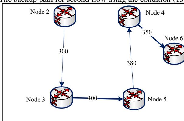
b – The backup path for second flow using conditions (14) only
