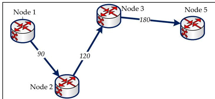
**Fig-4: The backup path for first flow using the condition (14)**
