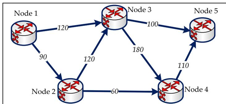
**Fig-1: The example of MPLS-network topology**
