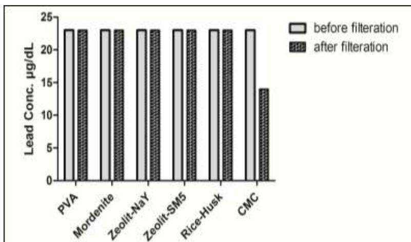
**Fig-2: Removal of Lead using different filters**
