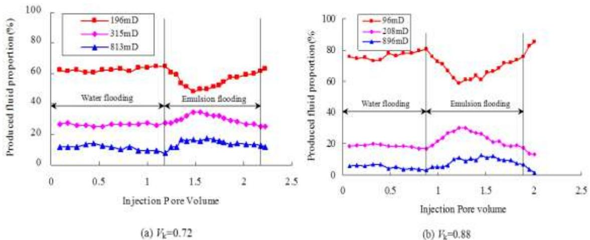
Fig-2: Produced fluid proportion curve of different permeability core
