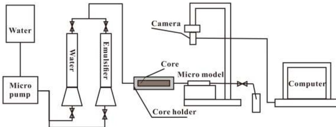
**Fig.1. Micro-displacement device used in experiment**
