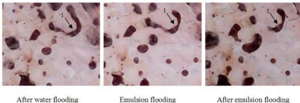
**Fig-4: The change of columnar residual oil during the emulsion flooding**
