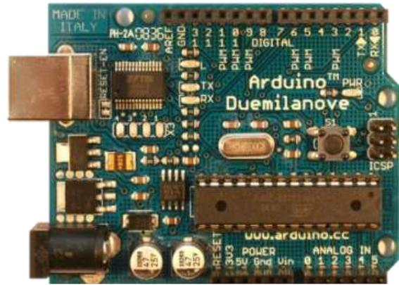
Fig- 5: Arduino Duemilanove A Tmega 328 microcontroller board
