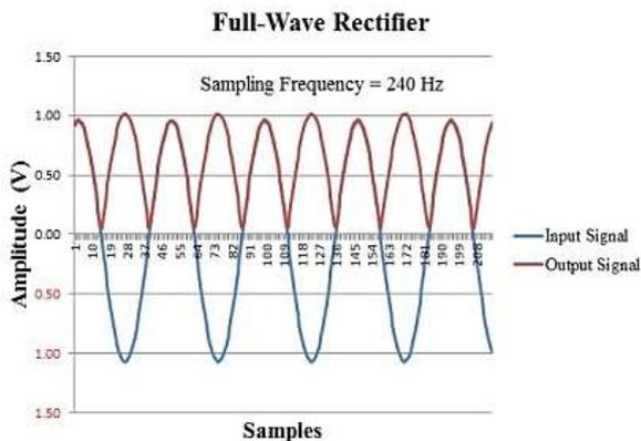
Fig-4: Full-wave rectifier input and output signals
