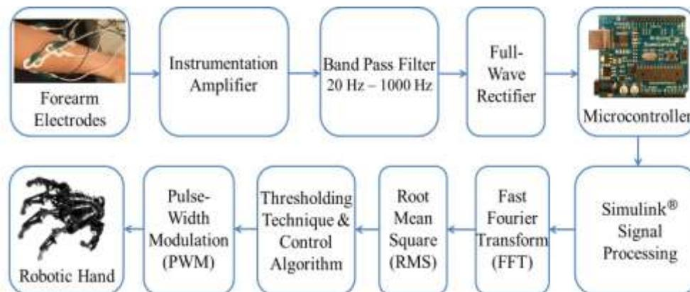
**Fig-15: Project flowchart depicting each step of the project. Acquiring the signal, processing the signal, microcontroller implementation, Simulink processing, and the final output of robotic hand movement**
