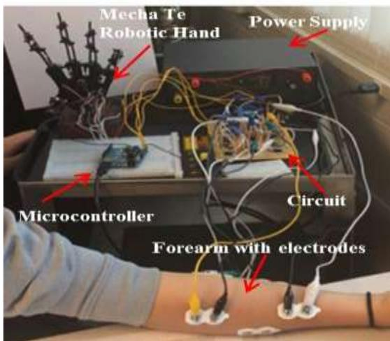
**Fig-8: Experimental setup with microcontroller, electrodes, and robotic hand.**
