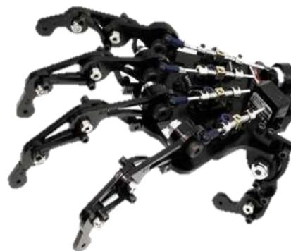
Fig-6: Mecha TE Hand with Futaba S3114 micro servos
