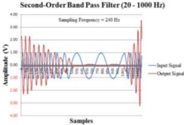
Fig-3: Band pass filter input and output signals
