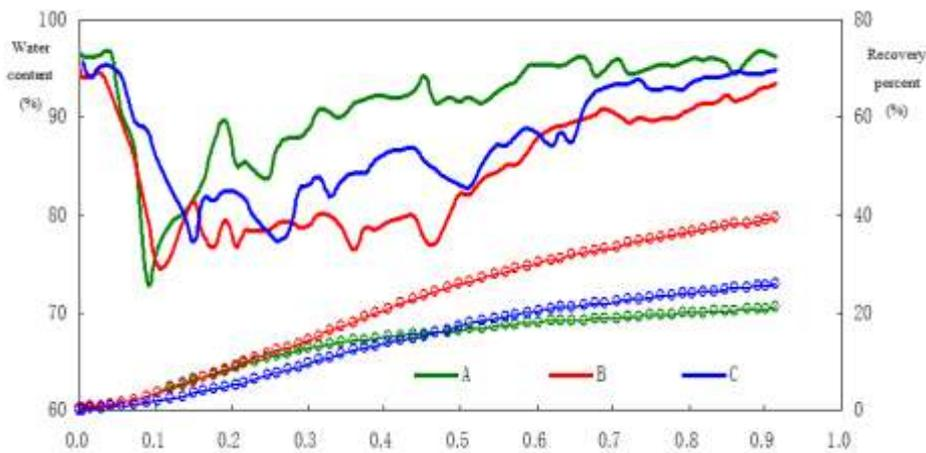
**Fig-3 Comparison of recovery percent and water content**
