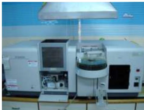
(b) Oil analysis instrument (Atomic absorption spectrometer)
