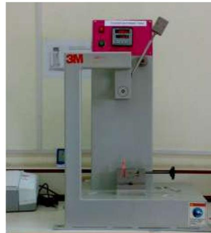
Fig-7 : Notched IZOD Impact Tester
