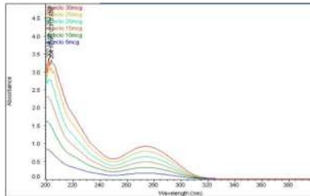
**Fig-3: Overlay spectrum of Aceclofenac(Zero order)**
