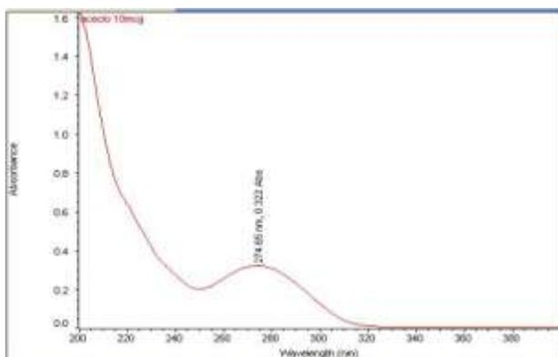
**Fig-2: Absorption maxima of Aceclofenac**
