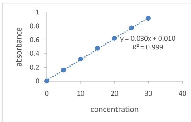
**Fig-4: Calibration curve of Aceclofenac(zero order)**
