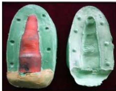
Fig.6: Stone flask with metal ring embedded in wax pattern and orientation grooves
