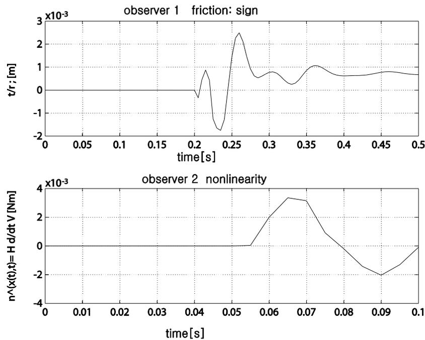
Fig. 4: Estimated nonlinear effects acting on the first motor(upper)and second motor(under)
