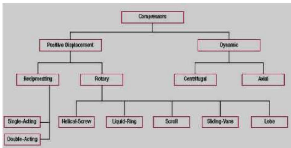
Fig-1: Types of Compressors (US DOE, 2003)
