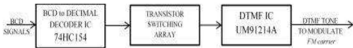
Figure 6: Block diagram showing level 3 description of how the control DTMF tones are generated
