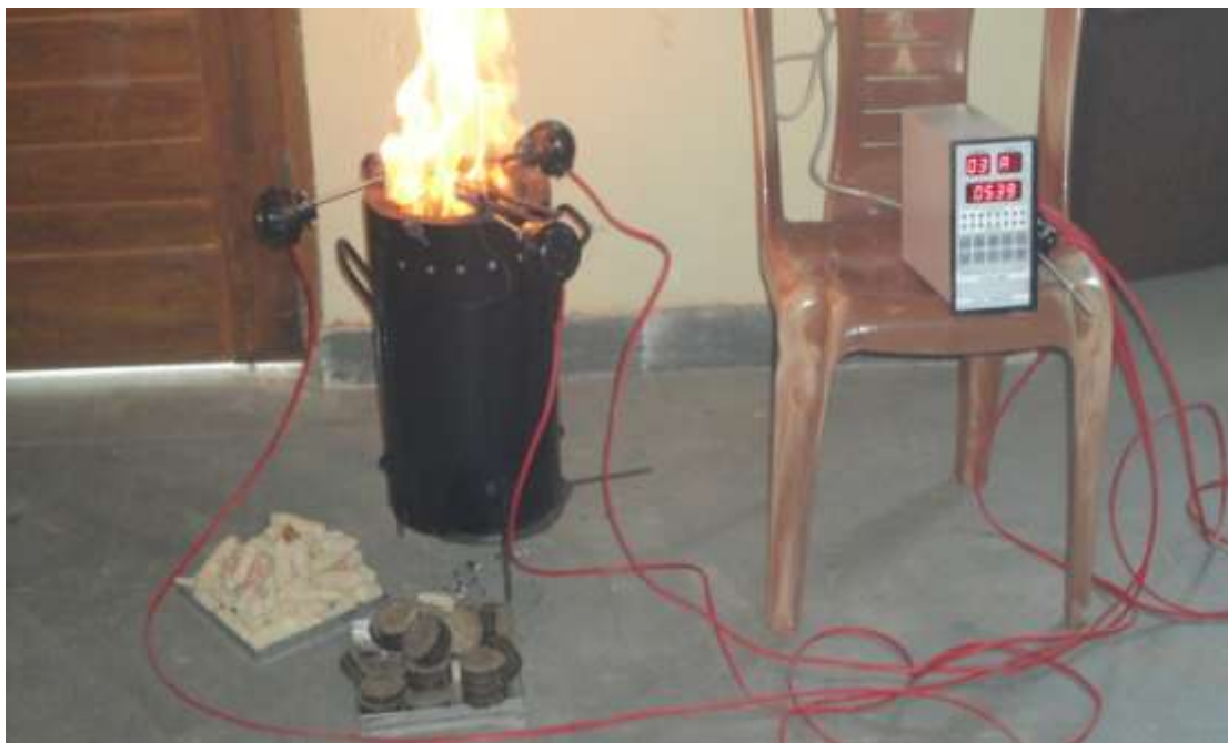
Fig- 2: Photographic Views of the Inverted Down Draft Gasifier
