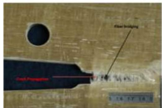
Fig. 15 Failure Mode of CT specimen
