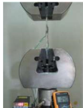
**Fig. 2 tension Specimen between the machines**
