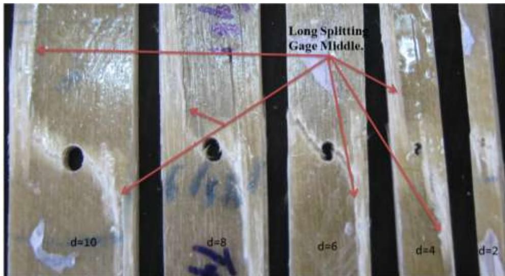
Fig. 29 Post failure image of [0, 45, 90, -45]<sub>s</sub>
