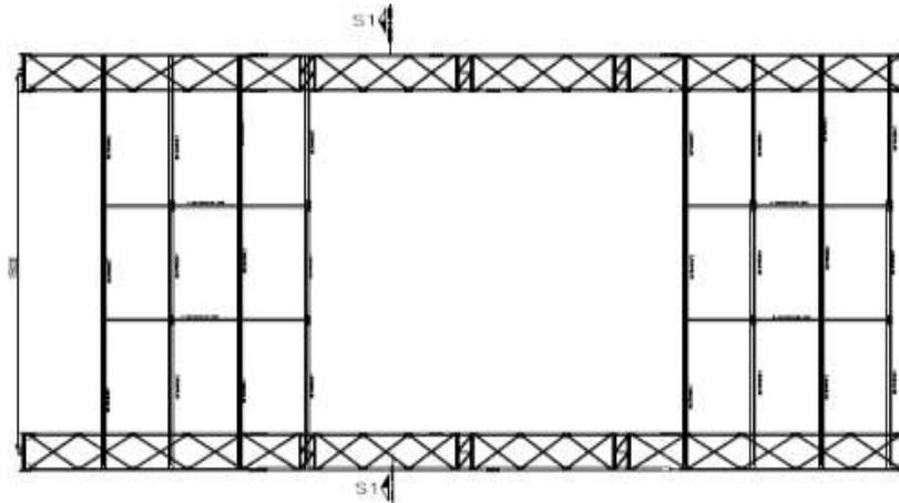
**Fig-7: Plan of PV mounting structure for typical 15 m span**
