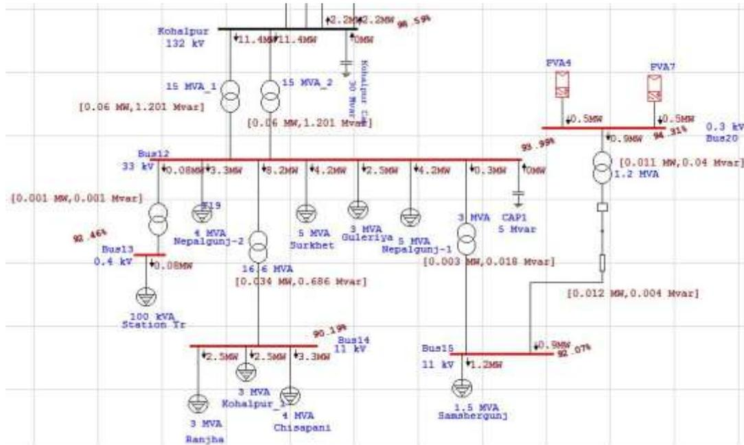
Fig-4: Load analysis of the grid after synchronization of solar PV
