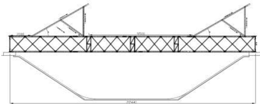
**Fig-6: Sectional view of canal along with PV mounting structure**
