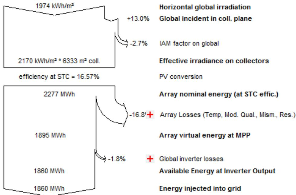
**Fig-2: Grid connected PV system losses diagram**
