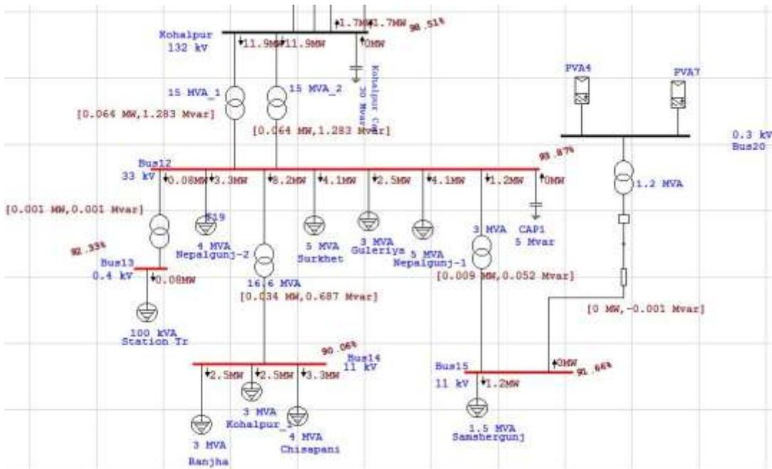
Fig-3: Load flow analysis of the grid before synchronization of solar PV
