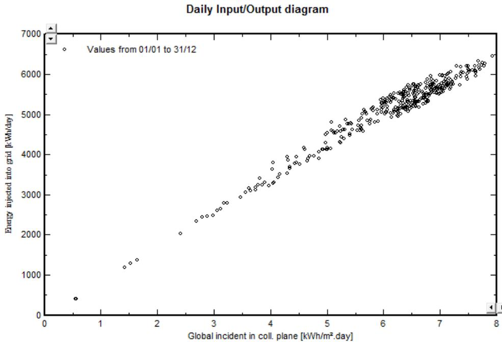
**Fig-1: Daily energy injected from 1MWp PV into grid as function of global solar incident**
