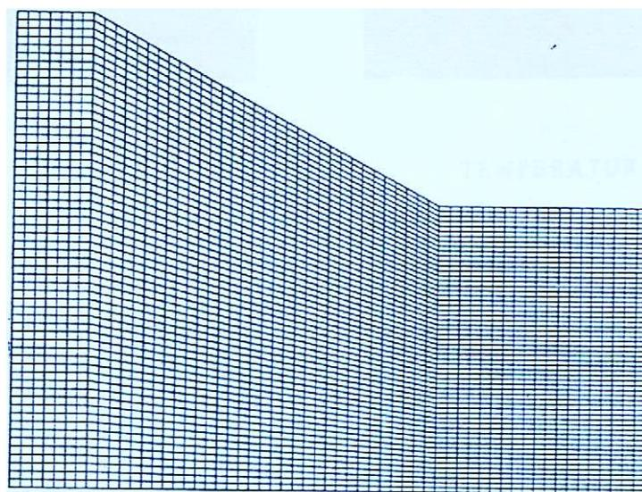
**Fig-2: Computational grid in the supersonic inlet**
