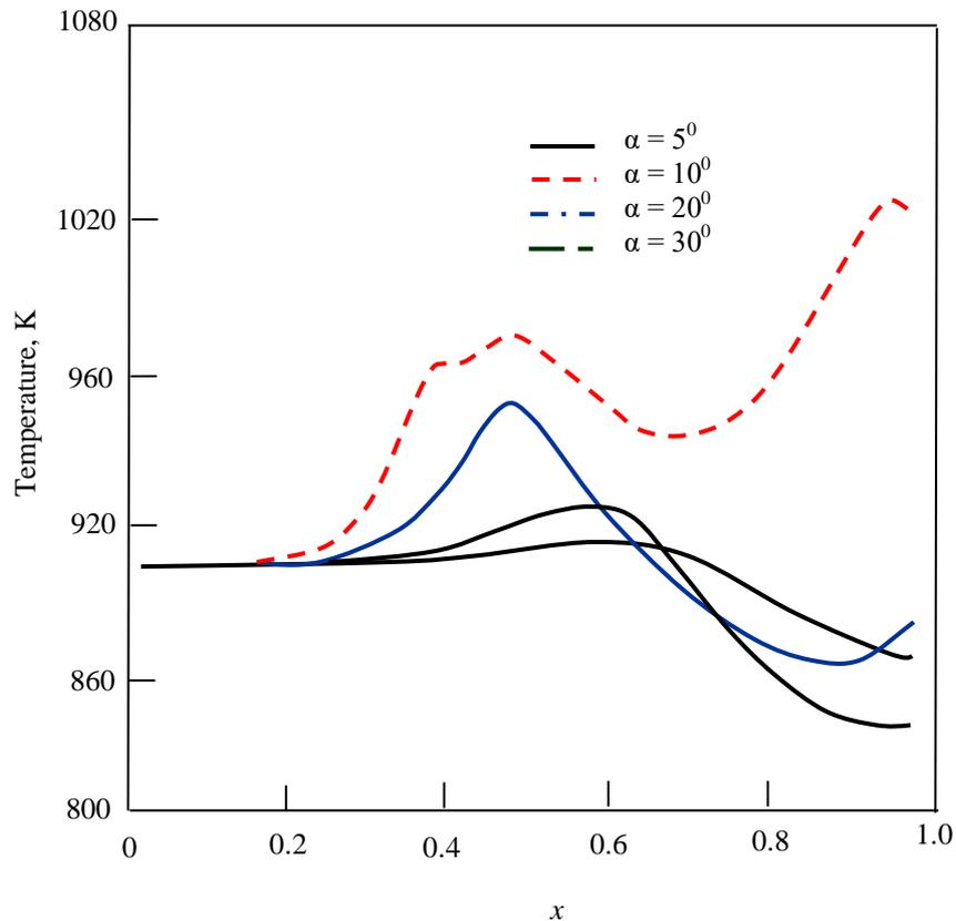
**Fig-7: Variation of temperature on lower wall of the inlet**
