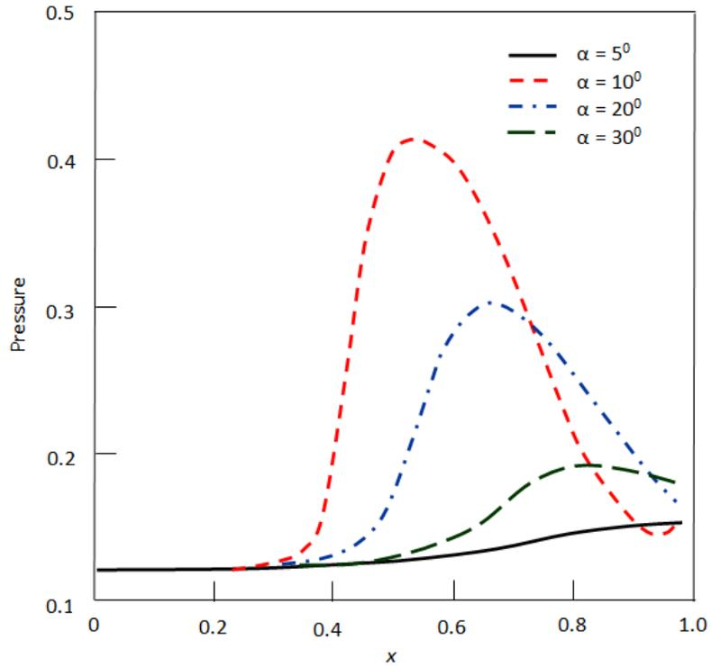
**Fig-5: Variation of pressure on lower wall of the inlet**
