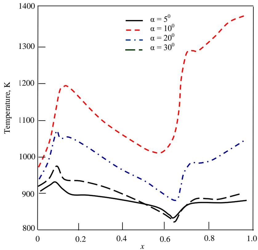
**Fig-6: Variation of temperature on upper wall of the inlet**
