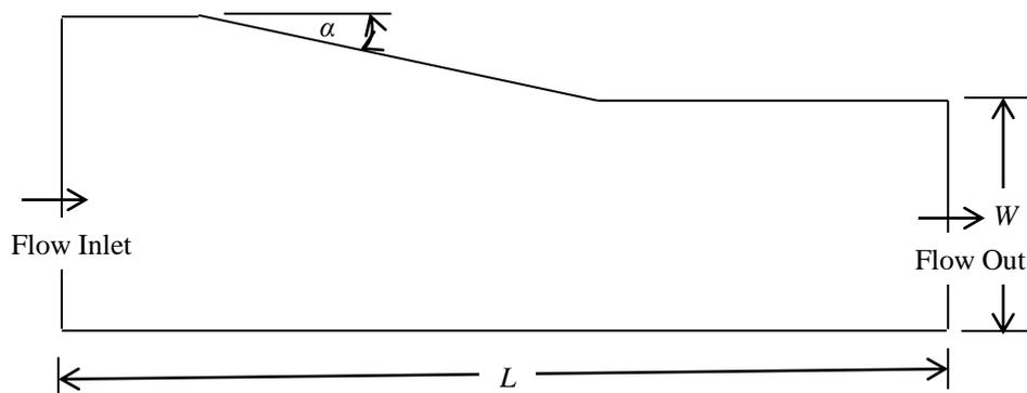
**Fig-1: Geometrical parameters of the supersonic inlet**
