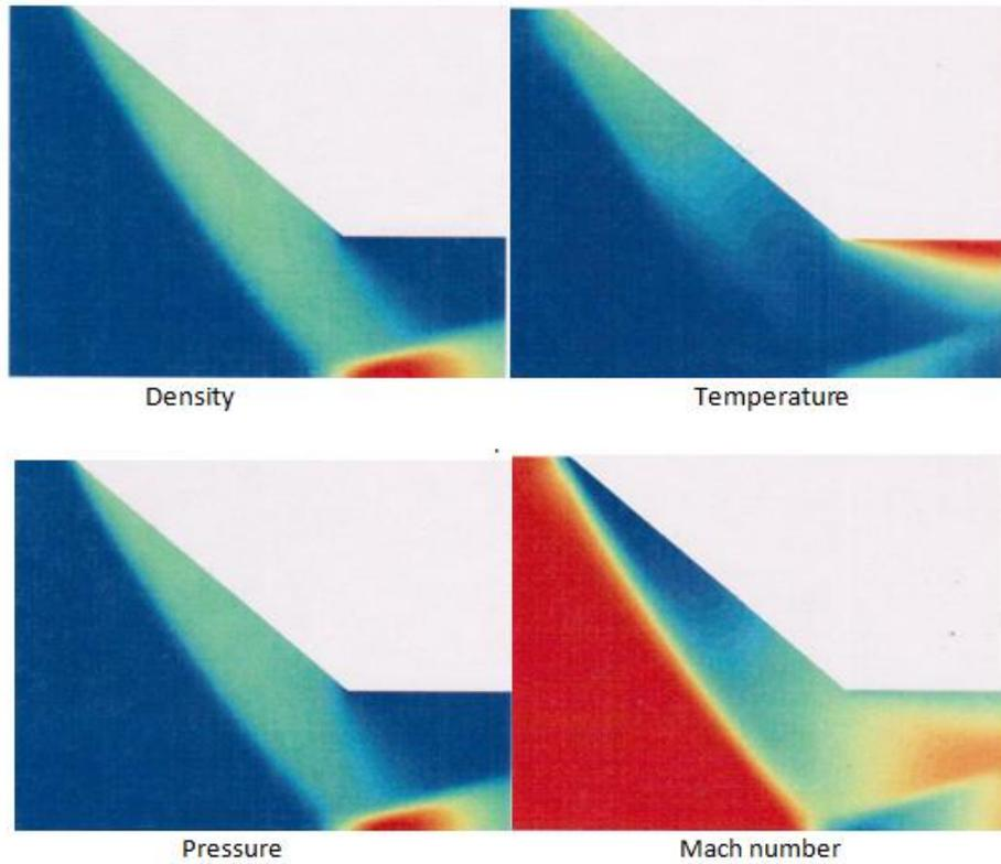
**Fig-3: Contour plots inside the supersonic inlet at  $\alpha = 20^\circ$**
